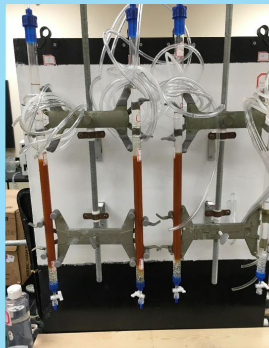
Figure 3: Bench-Scale Columns Housing Cation Exchange resin
