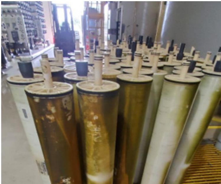
Old membrane elements with brown iron and sulfide deposits
