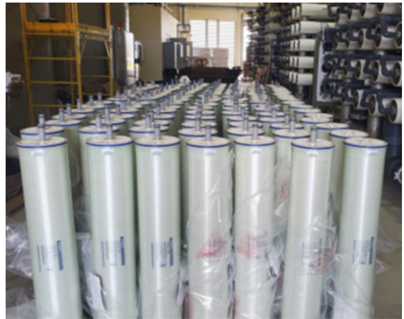
New membrane elements to be installed
